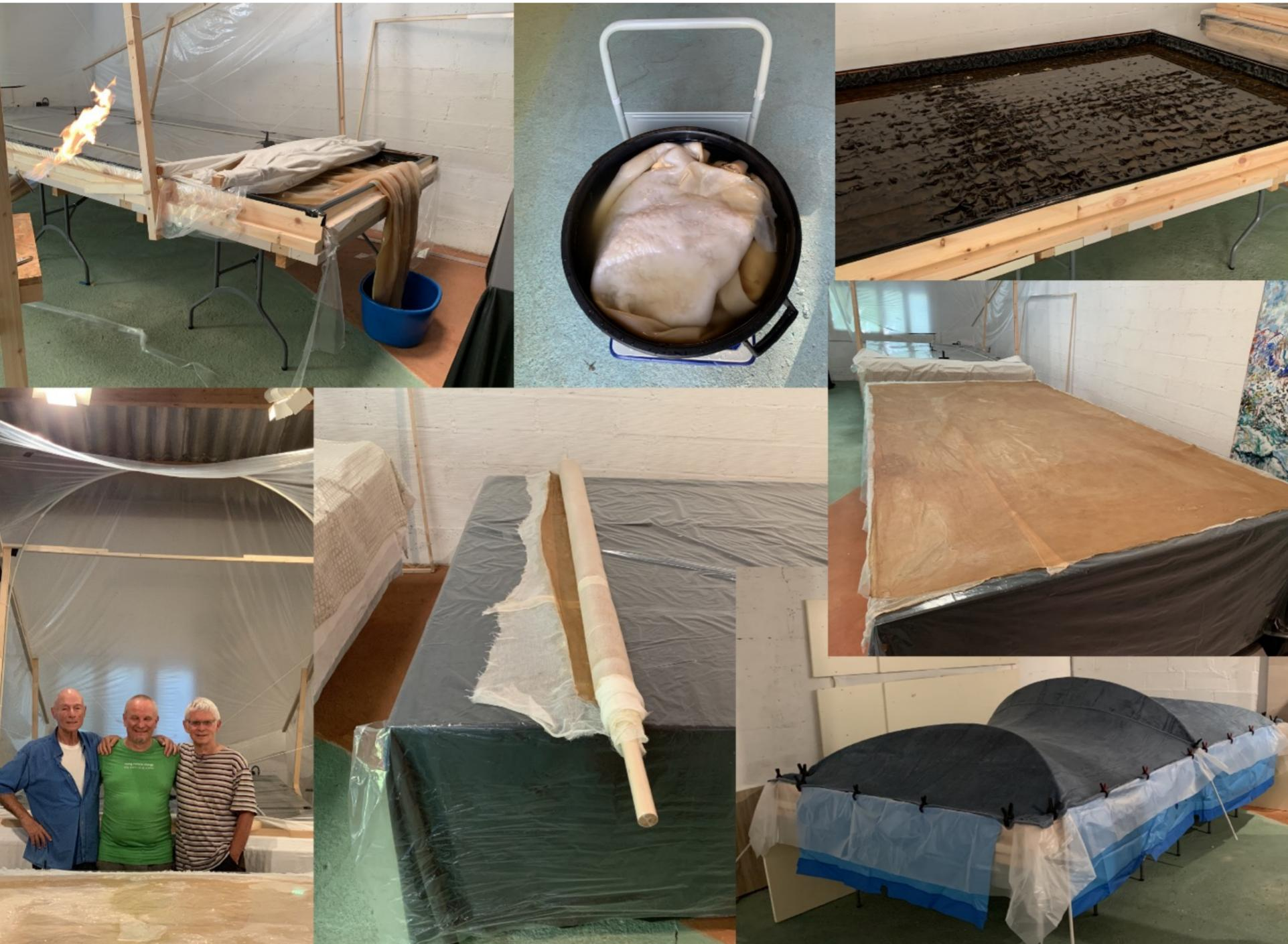
**EN** - The PAPUR pilot plant in Lalandusse, France operates 2 bioreactors that produce PAPUR leafs of 2 x 4 m size. Production is in monthly cycles of furbishing with fresh culture medium, incubation, harvesting PAPUR and refurbishing the reactor. The culture does not require human intervention in between. The PAPUR sheets are washed, dried, treated and stored as rolls. Depending on the season, the bioreactors get extra insulation and as need be a service & maintenance cycle.
